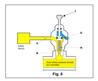
With the knob pressed downwards, in "check" position, the ways A and C are communicating, while way B is excluded. When the knob 1 is released, the communication between the ways A and B is automatically restored due to the tripping of the spring D.
