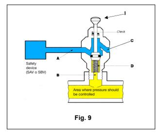
This valve is usually installed in the impulse line of safety devices against pressure increase and/or decrease (SAV or SBV) in order to be able to verify their calibrations in a very short time without disconnecting the impulse pipe during the periodic checks.
