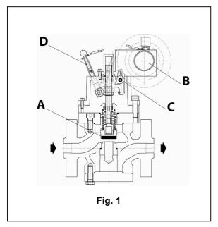
The pressure of the circuit to be controlled acts on the control head with a force opposing the forces of the setting springs for maximum and minimum pressure calibrated to the pre-set values.
