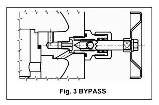
The release can be controlled also manually using the suitable button.
