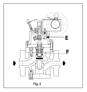
In order to restore the device, act on the lever **D** after having balanced the pressure on the obturator by feeding pressure through the manual bypass storage system with which the valve is equipped. After the restoration close the bypass.
