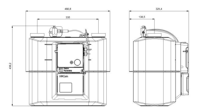
Fig.9 Overall dimensions HM25M, process connection 2"1/2 ISO 228-1
