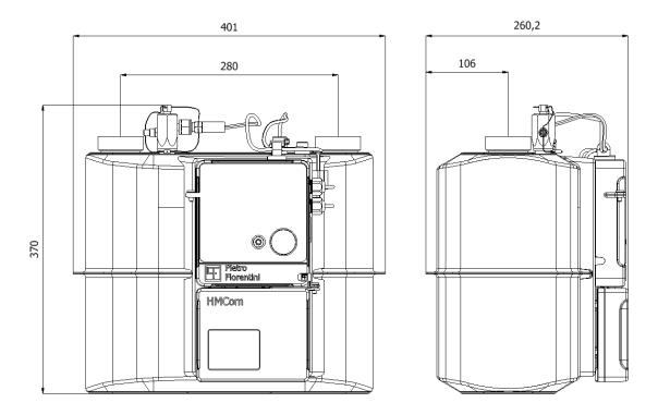
Fig.8 Overall dimensions of HM10M/16M, process connection 2" ISO 228-1
