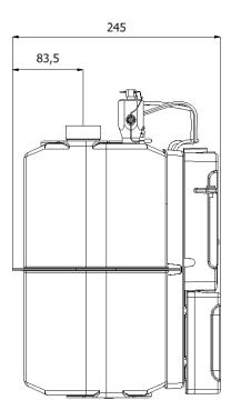
Fig.7 Overall dimensions of HM10M, process connection 1"1/4 ISO 228-1
