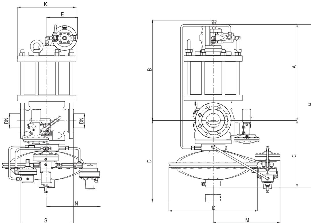
**Figure 9** Dimensions Terval/A + DB/93
