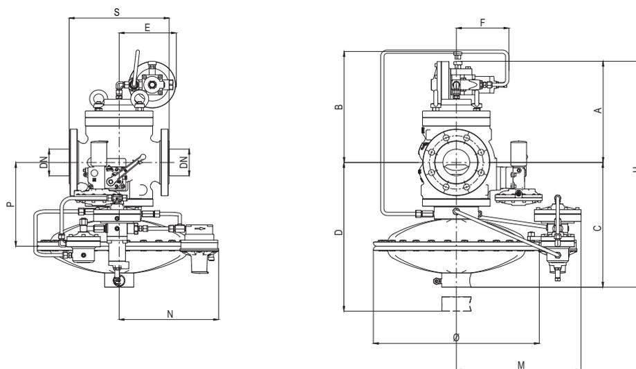
Figure 8 Dimensions Terval/A
